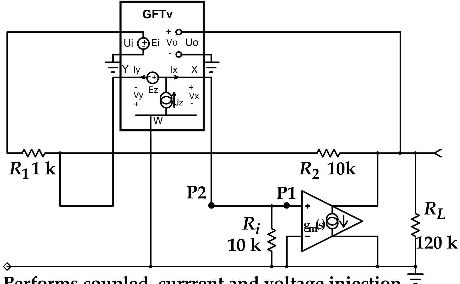
Performs coupled current and voltage injection
