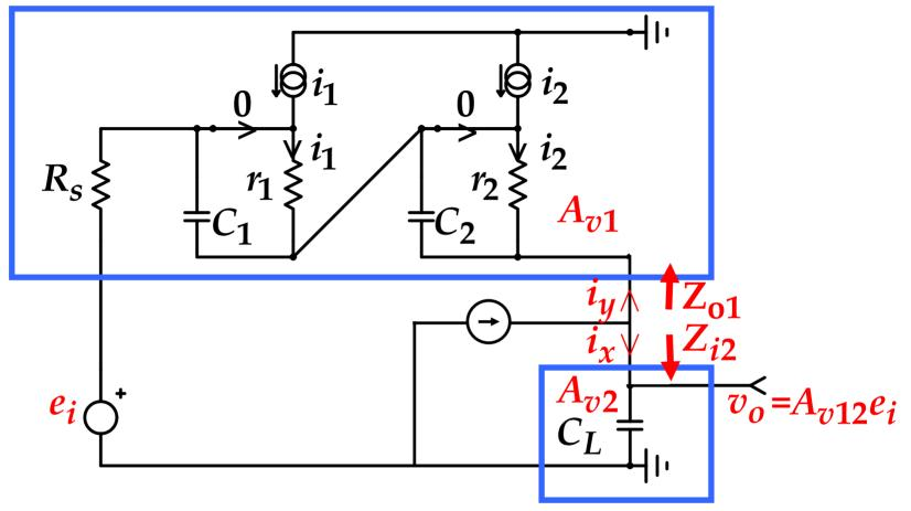
Nulled  $i_y$  means that the  $A_{v1}$  box is unloaded, so the input voltage to the
