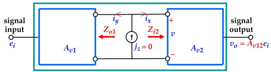
The gain  $A_{v12} \equiv \frac{v_o}{e_i}$  is given by the DT:  $A_{v12} = A_{v12}^{i_y} = \frac{1 + \frac{1}{T_{ni}}}{1 + \frac{1}{T_{ni}}}$
