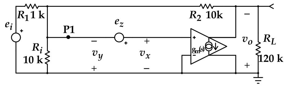
An ideal voltage injection point is where  $v_y$  comes from an ideal (zero impedance) voltage generator, or where  $v_x$  looks into an infinite impedance.
