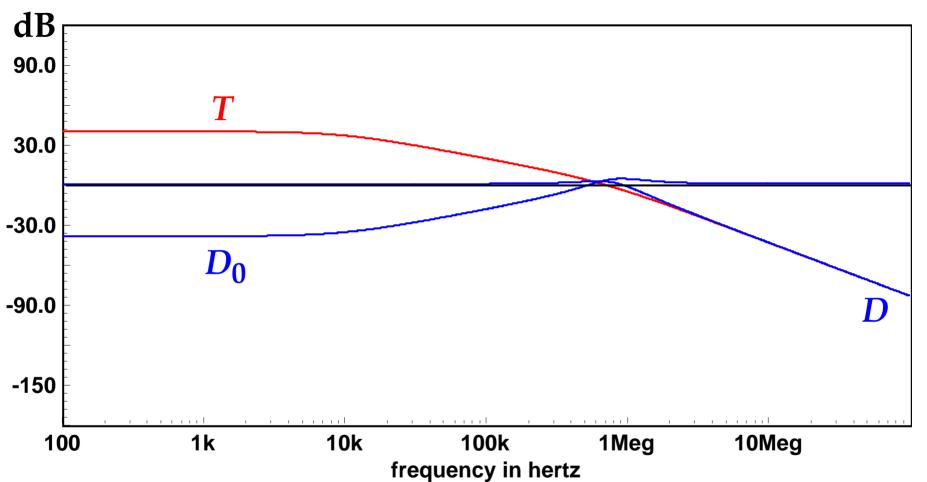
Design *T* to be large enough up to a sufficiently high frequency. Usually the most difficult step; includes
