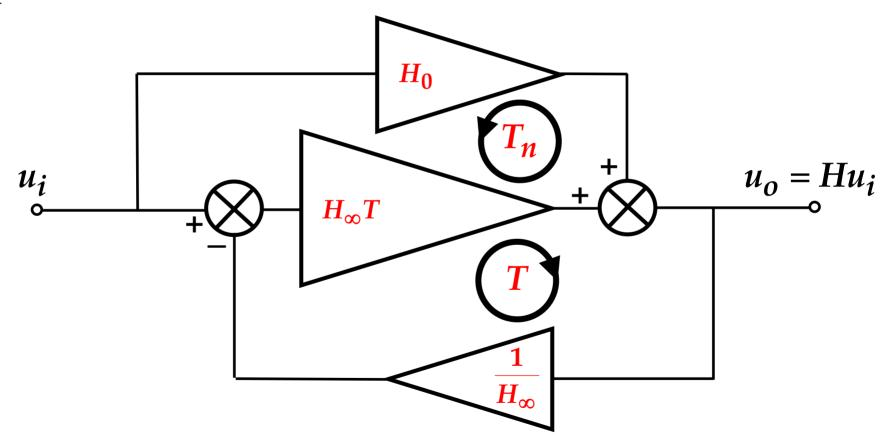
One of these nonidealities is the direct forward transmission through v.0.1.3/07 the feedback path "in the wrong direction."
