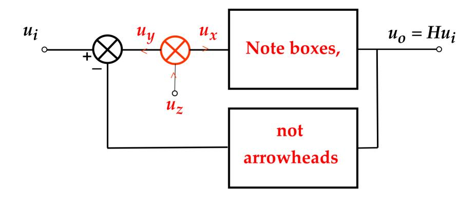
Inject a test signal  $u_z$  at error summing point. The GFT gives all the second-level TFs directly in terms of the circuit elements. As already seen, the GFT can be expressed as the weighted sum of two components:
