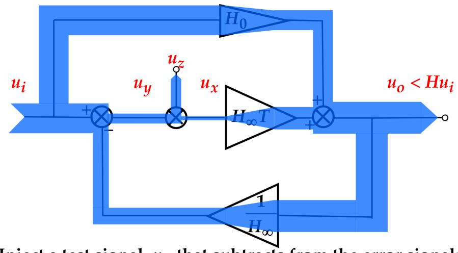
Inject a test signal  $u_z$  that subtracts from the error signal: the output  $u_o$  decreases and  $u_x$  decreases
