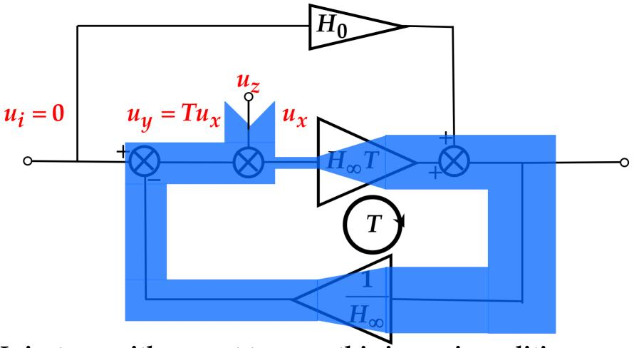
Inject  $u_z$  with  $u_i$  set to zero: this is an si condition.
