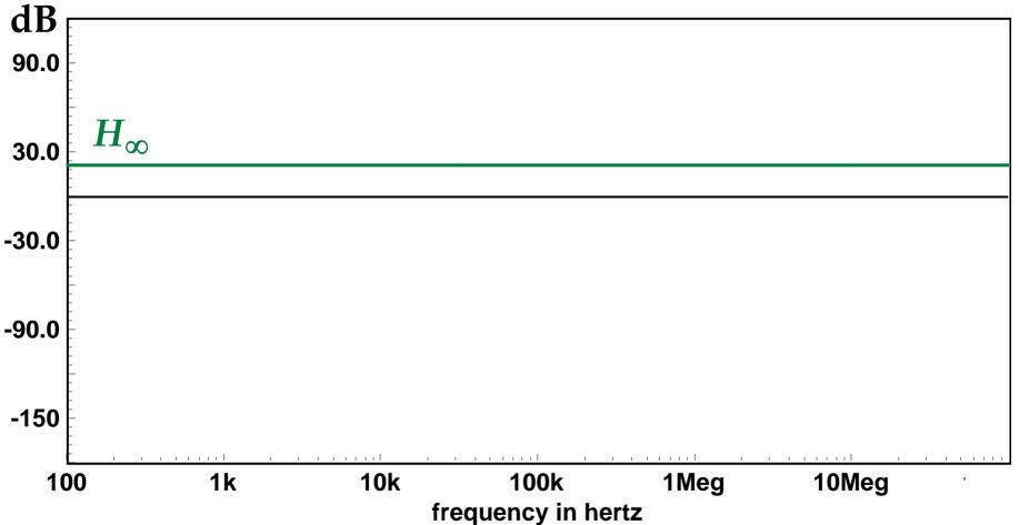
Design the feedback network  $K = 1/H_{\infty}$  so that  $H_{\infty}$  meets the specification
