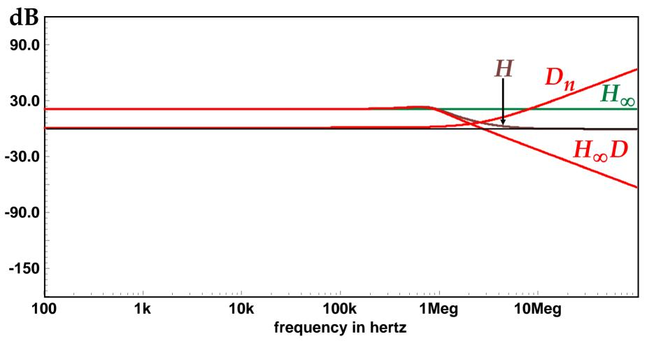
Construction of H with  $D_n$  as a multiplier term to  $H_{\infty}D$
