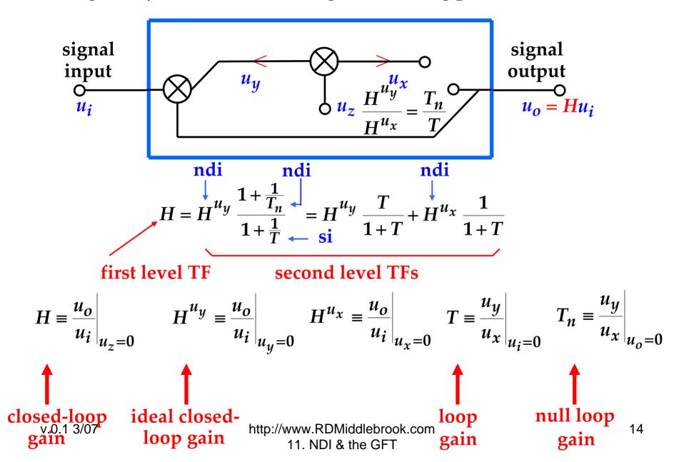
Test signal injection at the error signal summing point:
