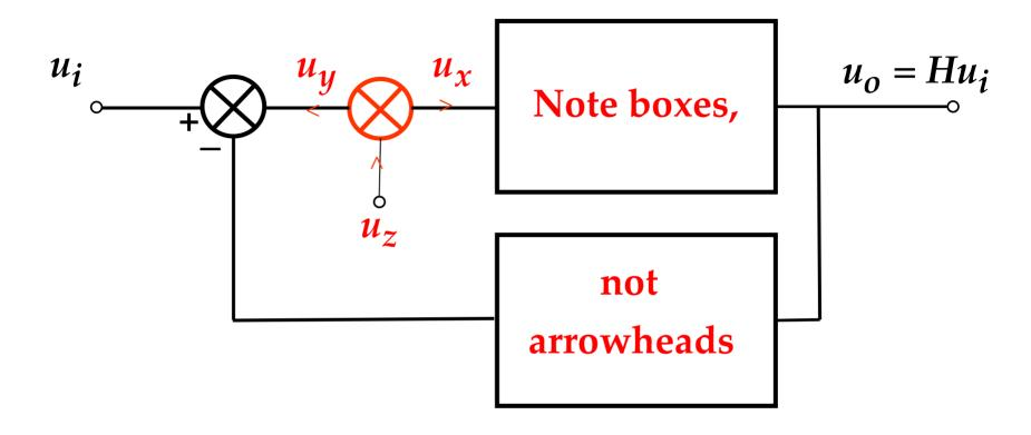
Inject a test signal  $u_z$  at error summing point. The GFT gives all the second-level TFs directly in terms of the circuit elements.
