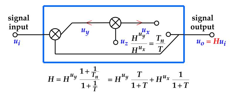
It is seen that the closed-loop gain *H* is the weighted sum of two components:
