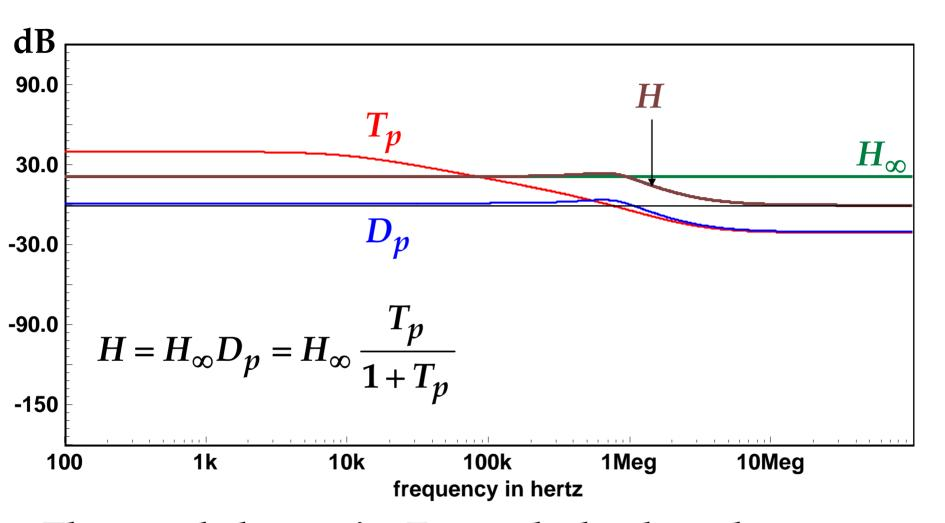
The pseudo loop gain  $T_p$  may be hard to relate to the circuit model, because it contains both T and  $T_n$  and  $T_n$  11. NDI & the GFT
