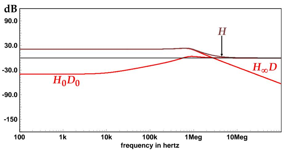
Construction of H with  $H_0D_0$  as an additive term to  $H_\infty D$
