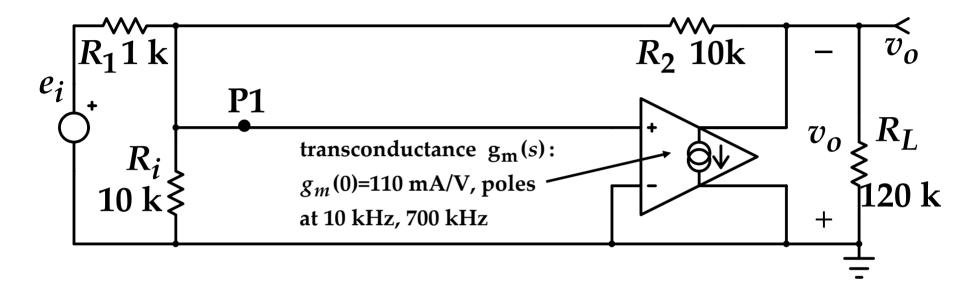
We want to get  $H_{\infty} = \frac{R_2}{R_1}$ , so inject  $e_z$  to add to the error voltage at P1:
