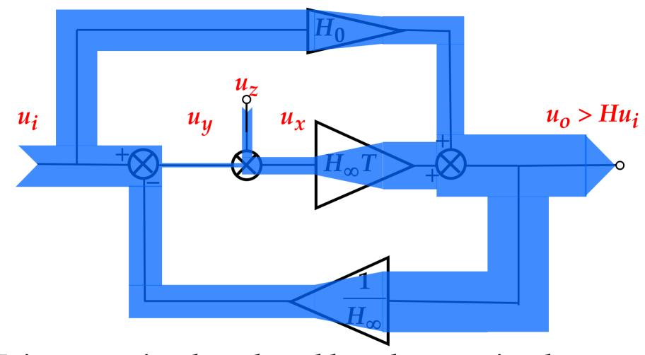
Inject a test signal  $u_z$  that adds to the error signal: the output  $u_o$  increases and the error signal  $u_y$  decreases
