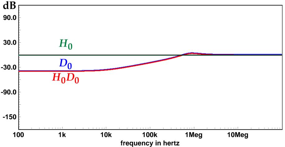
Design the direct forward transmission so that  $H_0$  is small enough that the actual H meets the
