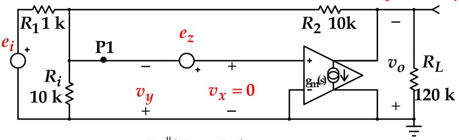
$$H^{v_x} = \frac{R_L}{R_2 + R_L} \frac{R_i \| (R_2 + R_L)}{R_1 + R_i \| (R_2 + R_L)} = 0.83 \Rightarrow -1.6 \text{ dB}$$
