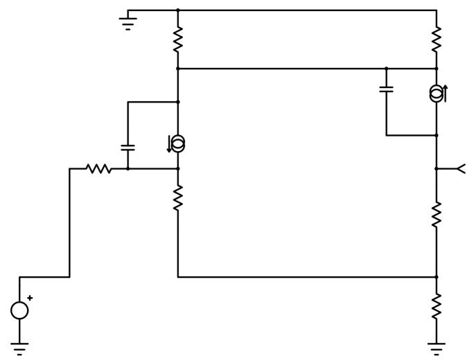
If the second device fails open, the input signal can still reach the output by going the "wrong way" thirty graphic feedback path.
