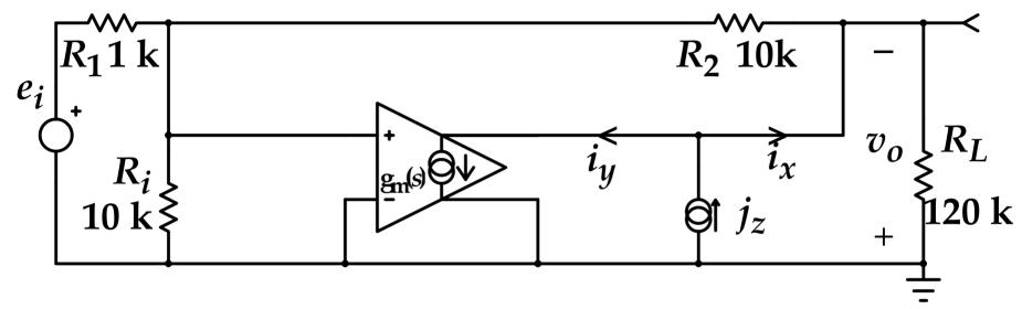
An ideal current injection point is where  $i_y$  comes from an ideal (infinite impedance) current generator, or where  $i_x$  looks into a zero impedance.
