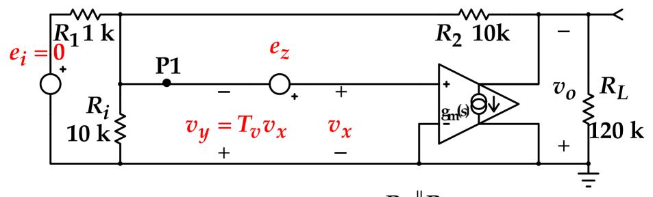
$$T_v(0) = g_m(0)[R_L \| (R_1 \| R_i + R_2)] \frac{R_1 \| R_i}{R_1 \| R_i + R_2} = 92 \Rightarrow 39.2 \text{ dB}$$
