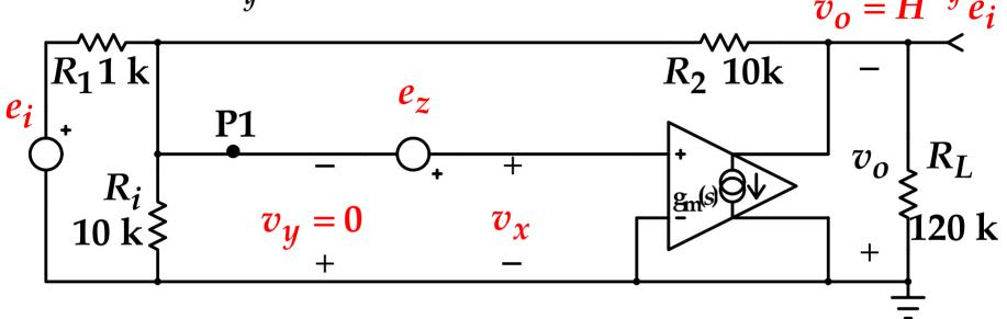
$$H^{v_y} = \frac{R_2}{R_1} = 10 \Rightarrow 20 \text{ dB}$$
