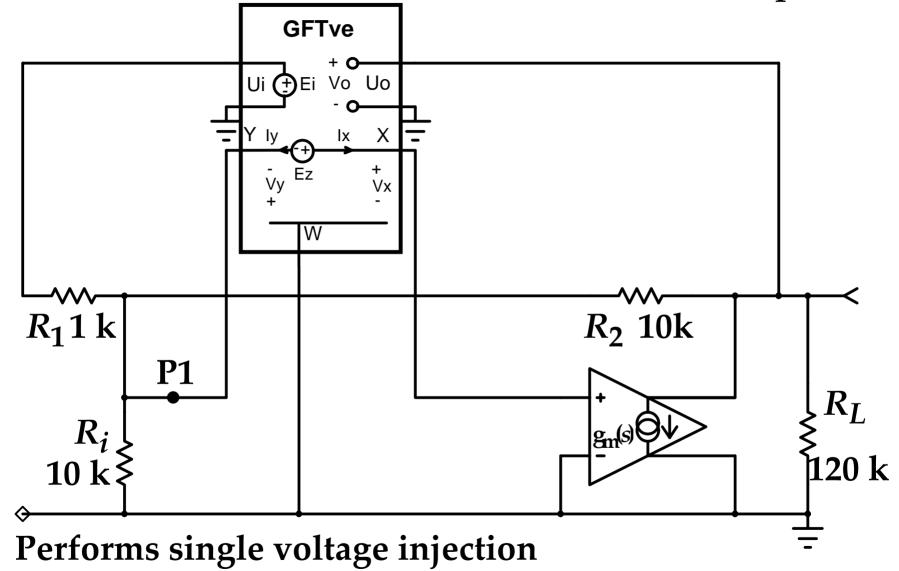
The GFT Template calculates all the second-level TFs  $H_{\infty}$ , T,  $H_0$ ,  $T_n$  and inserts them into any version of the first-level TF H, for comparison with the directly calculated H (the "normal" closed-loop gain with no injected test signal).
