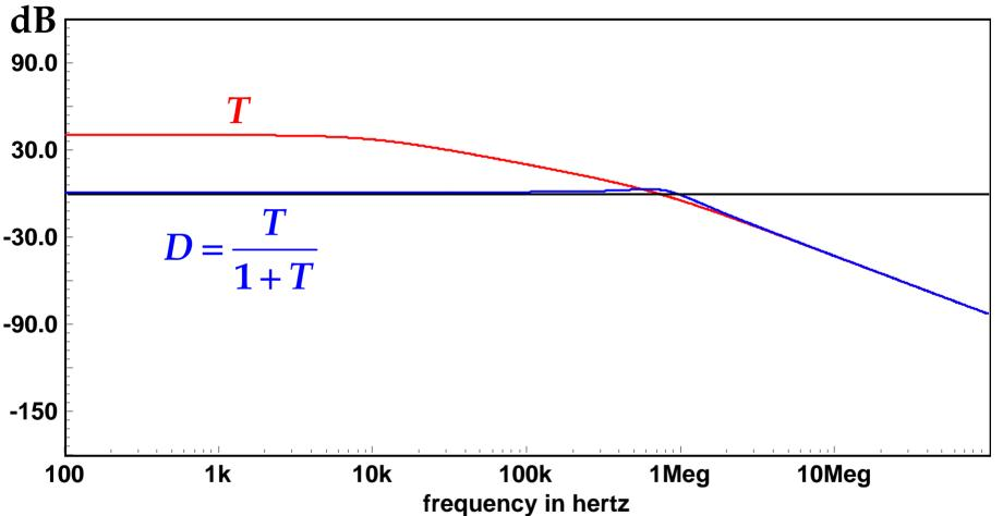
Design the loop gain so that T is large enough that the actual H meets the specification within the
