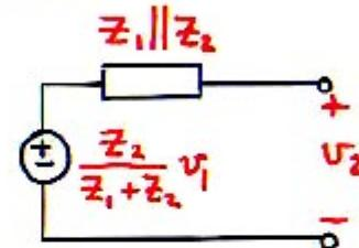
Every time Norton's theorem is used, one node is removed from the circuit:
