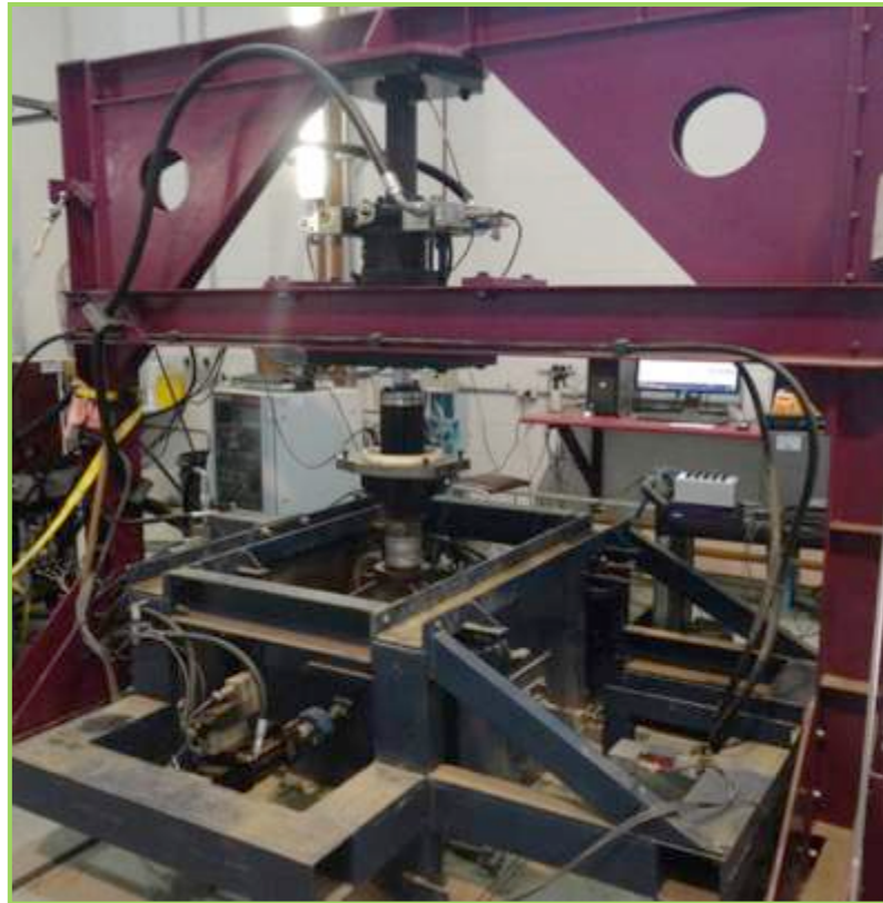
Cubical Triaxial Apparatus to Simulate a Track Section (Specimen: 800x600x600 mm)
