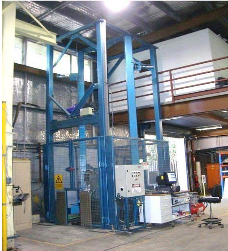
High capacity drop weight Impact test Apparatus
