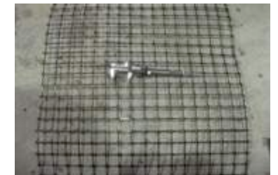
Biaxial Geogrid Aperture size = 40mm
