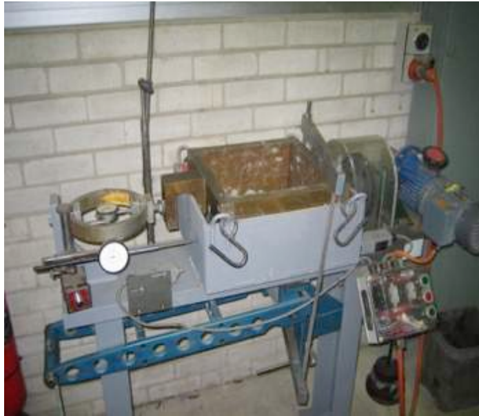
Large-Scale direct shear box Dimension: 300x300x200mm
