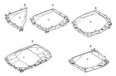
only half the crystal is present in nature and that the left half, the point of attachment being near the symmetry plane. This development is very constant and by being familiar with it one can recognize the prominent faces at a glance.
