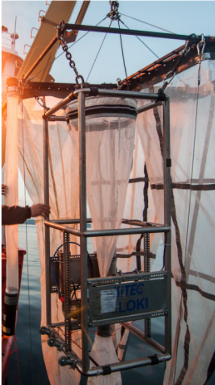
Figure 7: LOKI attached to a 5-Net Vertical Sampler. Photo credit: Jessy Barrette
