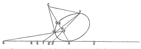
Construct two points D, D' on the tangent at A, having no connection with the particular  $CP_1$  or  $CP'_1$  or  $CP'_1$  as follows. On COA, which meets UV in G, take E the harmonic conjugate of C with regard to O, G, and Feither double point of the involution of which C, E and A, G are pairs. D and D' are where FU and FV meet the tangent.
