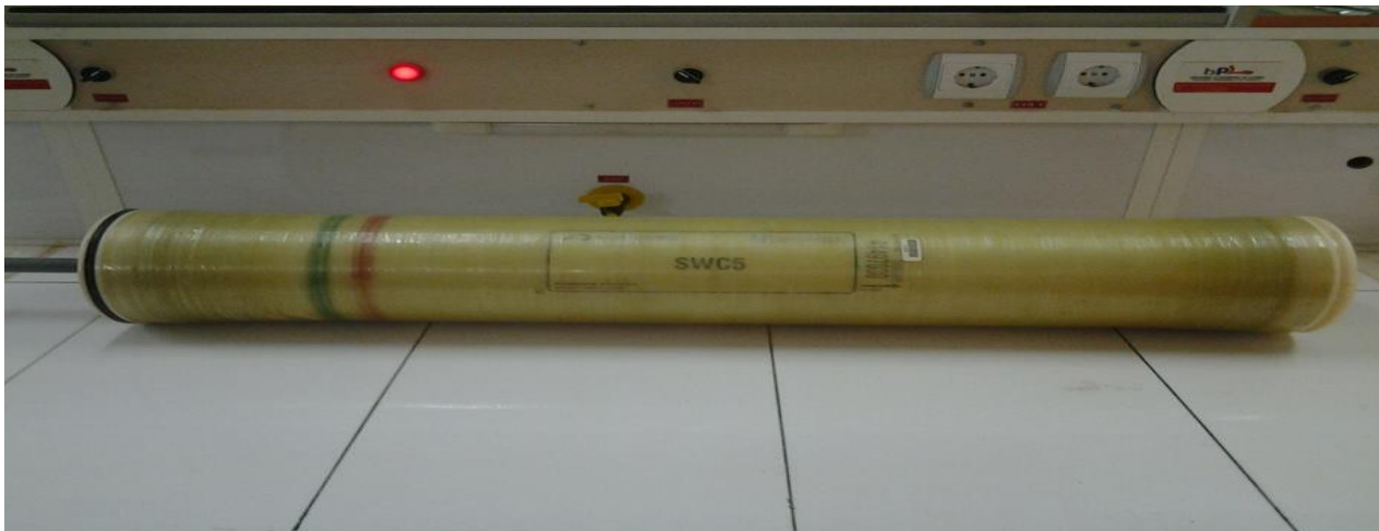
Fig. 2: The fouled RO membrane element
