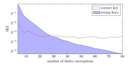
Fig. 7. SEI values for correct key ( $SEI_c$ ) plotted against best SEI for a wrong key ( $max(SEI_w)$ ) for increasing number of faulty encryptions. Setup: AES software implementation, single clock glitch.
