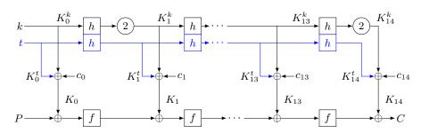
Fig. 6. Block cipher Deoxys-BC-256.
