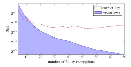
**Fig. 9.** Evolution of the SEI values with increasing number of faulty encryptions. Setup: AES hardware co-processor of a smartcard microcontroller, laser.
