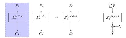
Fig. 5. Plaintext processing for Deoxys $^{\neq}$ .
