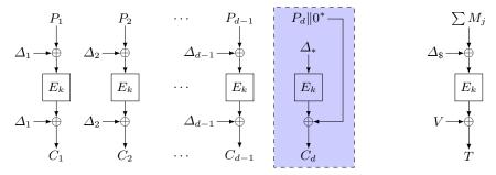
Fig. 3. Encryption in OCB.
