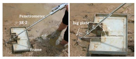
Figure 1 Penetrometer and penetrometer frame, penetration resistance measurement method
