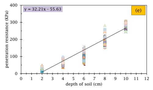
Figure 5 Graph of soil depth vs pressure resistance (a) pressure angle 30° (b) pressure angle 45° (c) pressure angle 60° (d) pressure angle 75° (e) pressure angle  $90^{\circ}$
