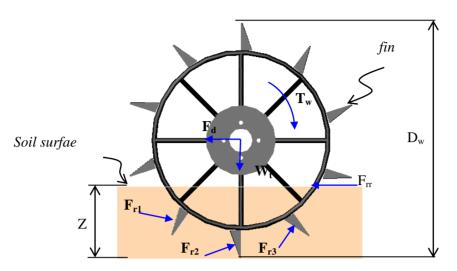
Figure 2 A force scheme that acts on the cage wheel for wheel design parameters
