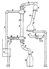
accordingly. It is well to make sure, however, that the diameter of this pipe, and the rate of flow of the water in it, are sufficient to insure condensation in the tube H.
