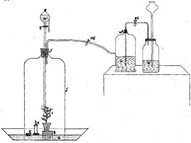
From the diagram, it will be seen that I aimed to give my plant all the constituents of ordinary air and earth, and all other conditions, i. e., N<sub>2</sub>, CO<sub>2</sub>, NH<sub>3</sub> (traces), H<sub>2</sub> O, sunlight and heat, but NO OXYGEN. That part of the apparatus marked B furnished the CO<sub>2</sub>, of which I let in a small number of bubbles each day. The wash bottle prevented any H Cl fumes to get into J.
