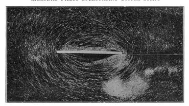
Fig. 11—Strip Carrying 107 Amperes at 838 ~ A-C.
