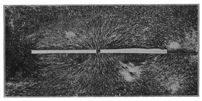
Fig. 12—Outgoing and Return Strips Carrying 120 Amperes at  $858 \sim \text{A-c.}$
