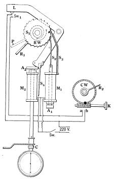
FIG. 6-ELECTROMAGNETIC REVOLUTION COUNTER
