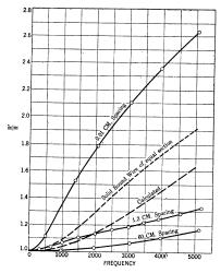
FIG. 17—WHOLE COPPER TUBE— OUTSIDE DIAMETER 1.266 CM., WALLS 0.159 CM.
