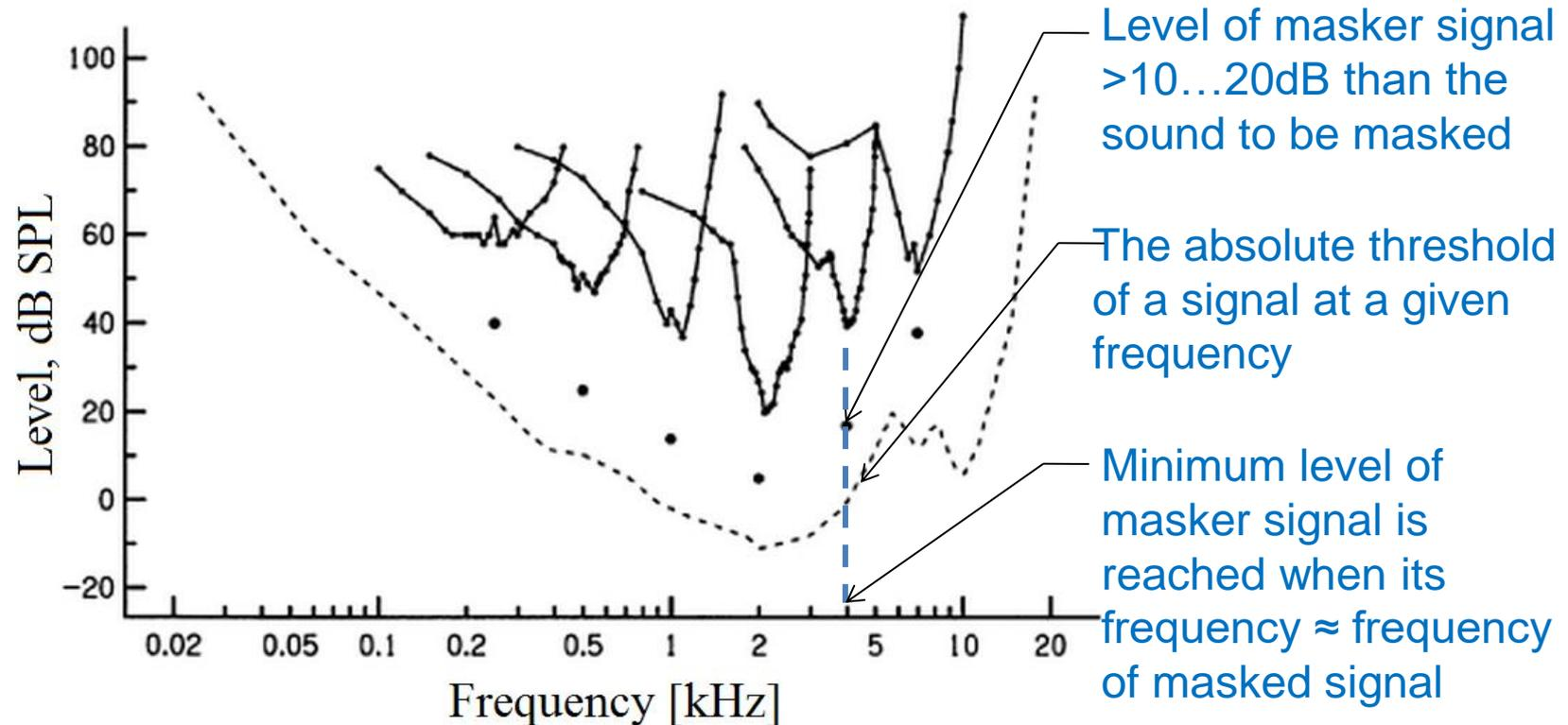
Fig.2-Measurements of psychophysical tuning curves showing the level of masker signal which is needed to successfully mask a signal of a given frequency [1]
