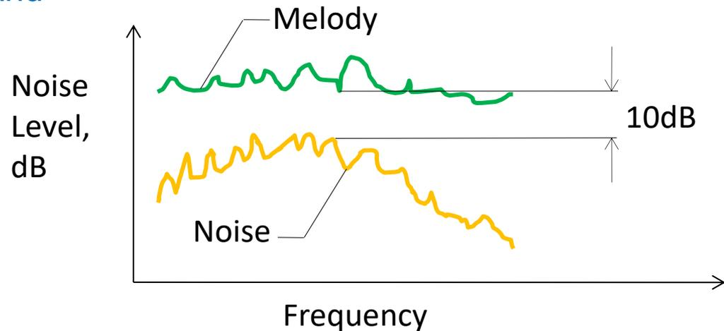
**Fig.8- Scheme showing how emitting of a melody can mask the broad band noise**
