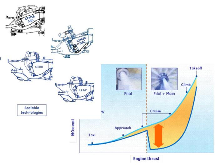
Controlling temperature with Lean-Burn is key to minimizing NOx: the TAPS combustor will provide even more significant reductions as shown in Figure during high altitude climb and cruise conditions, where approximately 90% of NOx emissions are emitted. FORUM-AE assessment against ACARE emissions goals
