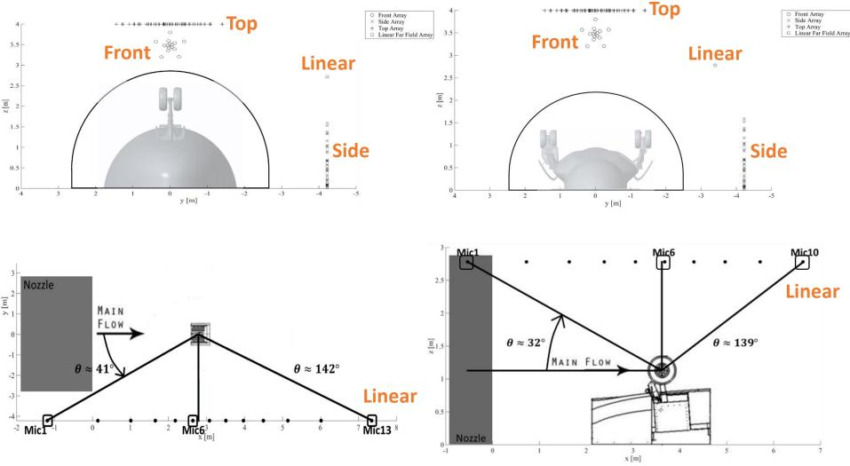
Diagram of linear far field array angles for the NLG
