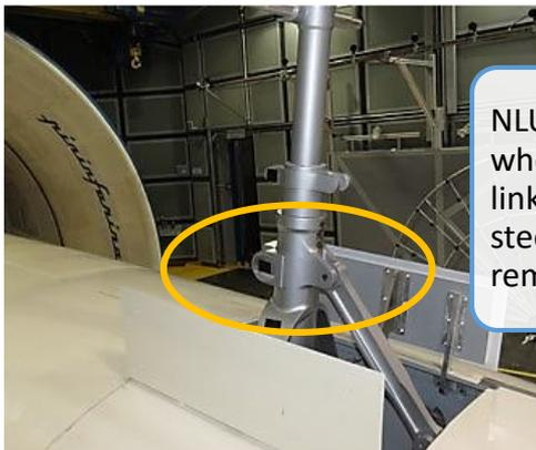
NLU with wheels, torque link and steering pinion removed
