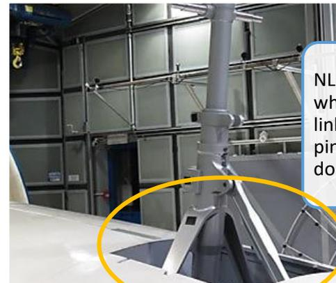
NLU with wheels, torque link, steering pinion and doors removed
