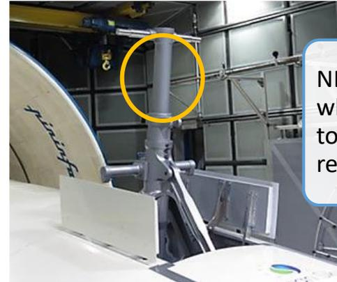
NLU with wheels and torque link removed
