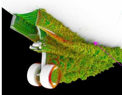
L.G. noise is strongly reflected by fuselage
