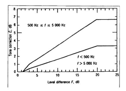
Level-difference (F) is transformed into a tonal correction factor (C) depending on the third-octave frequency band.
