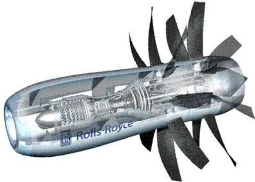
Courtesy of Rolls-Royce plc - Advanced open rotor concept
