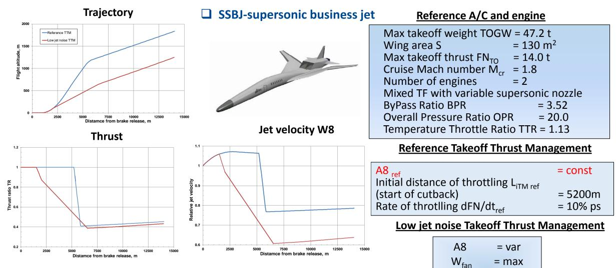
significant lowering of trajectory above the flyover point due to thrust reduction
