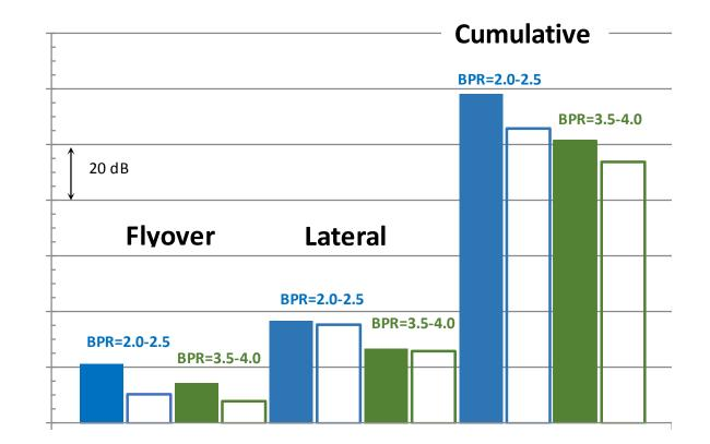
Impact on jet noise at takeoff for different BPR engines
