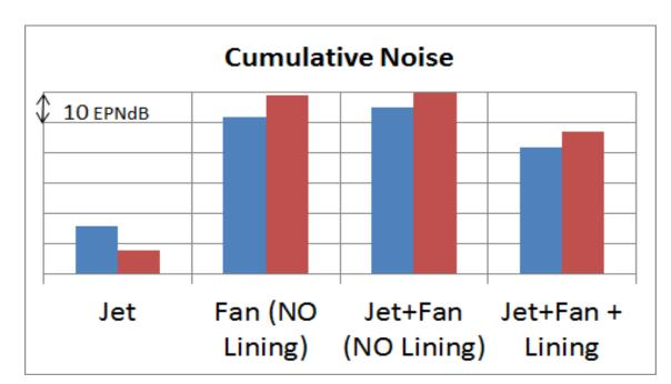
Prediction of total aircraft noise (taking into account jet and fan noise and use of acoustic liners) showed that Low Jet noise Takeoff Thrust Management vs Reference TTM is higher by 5 EPNdB.
