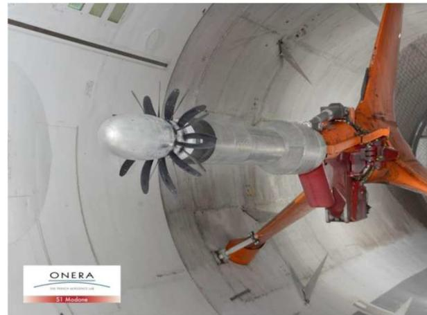
Tests in ONERA's S1MA transonic wind tunnel
