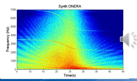
Mid range aircraft take-off measured at microphone below flight path
