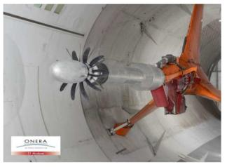
Tests in ONERA's S1MA transonic wind tunnel
