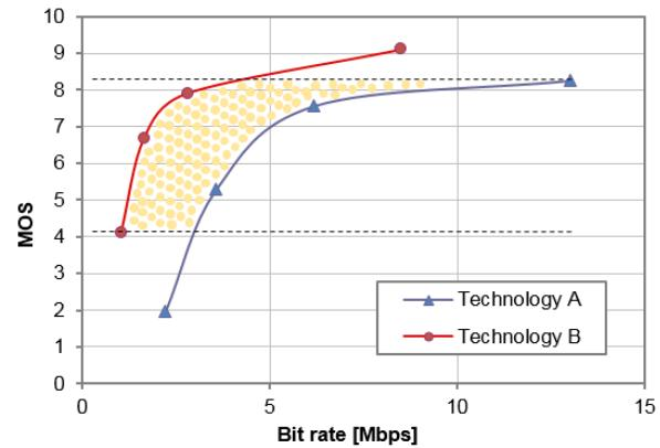
Figure 1 – Example quality interval used in BD-rate computation.
