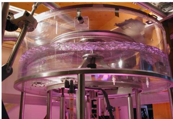
**Figure 1:** Small annular wind-wave facility (construction Erik Bock) used for the experiments.
