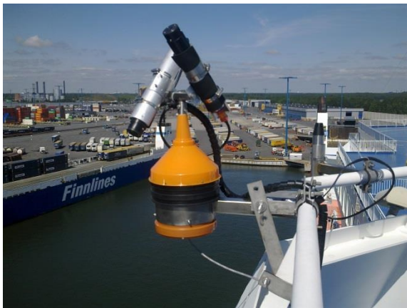
Figure 2 (left) Spectroradiometers on a low-cost azimuth controller on a Baltic Sea ferry by the Finnish Environment Institute. (right) The Sea-bird scientific SAS solar tracker.
