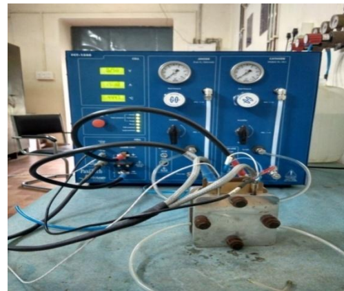
Fig. 1. Biologic FCT 150S PEM fuel cell setup
