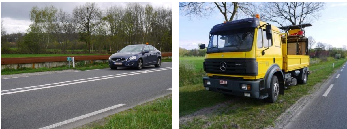
Fig. 8 VOLVO S60 passenger car (left) and Mercedes 1827 lorry used for the CPB measurements
