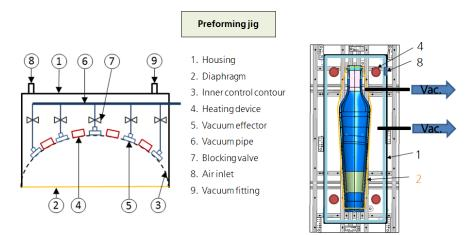
Fig. 9: Design of the compacting unit [3]
