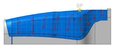
Fig. 4: Principle of the manual draping process, as an illustration of the force application steps
