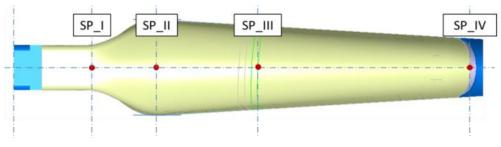
Fig. 2: Predefinition of four possible initial draping points on the top of the tooling
