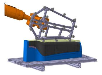
This process requires a rolling movement of the end-effector on top of the tooling.
