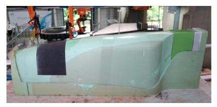
Fig. 1: Male AFS Tooling used for the development of an automated preforming process
