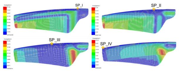
Fig. 3: Shearing effects based in location of initial draping point [1]
