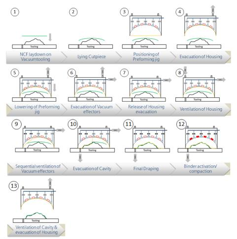
Fig. 10: Sequence of the automated drape and compacting process [3]
