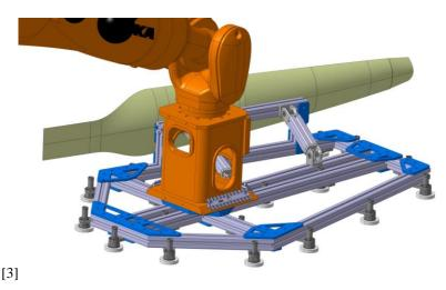
Fig. 6: Transport and deposition end-effector [3]
