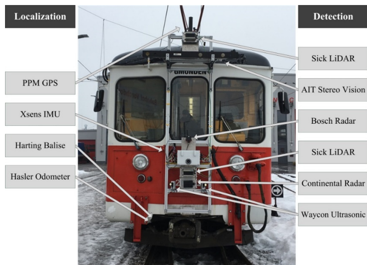
Fig. 2 demonstrator train used for field tests
