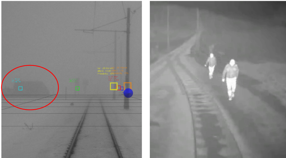
Fig. 3 (a) radar sensor with dense fog and crossing car; (b) IR camera and pedestrian
