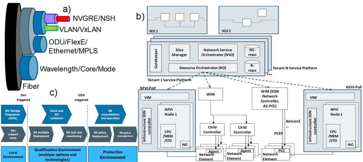
**Figure 1. a) Optical Network Virtualization, b) Proposed Network Slicing architecture; c) DevOps for Networking lifecycle**
