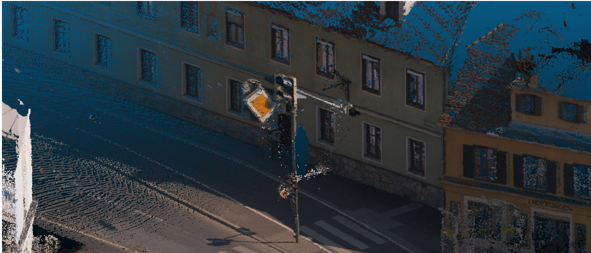
Fig. 4 Errors due to parallax when warping LiDAR points captured after the colour images back to a common trigger point. The street sign and the traffic light in the foreground are projected onto the facade in the background. Additionally, artefacts from the densification step can be seen as points scattered between the facade in the background and the post in the foreground. The effect has been exaggerated for visualization
