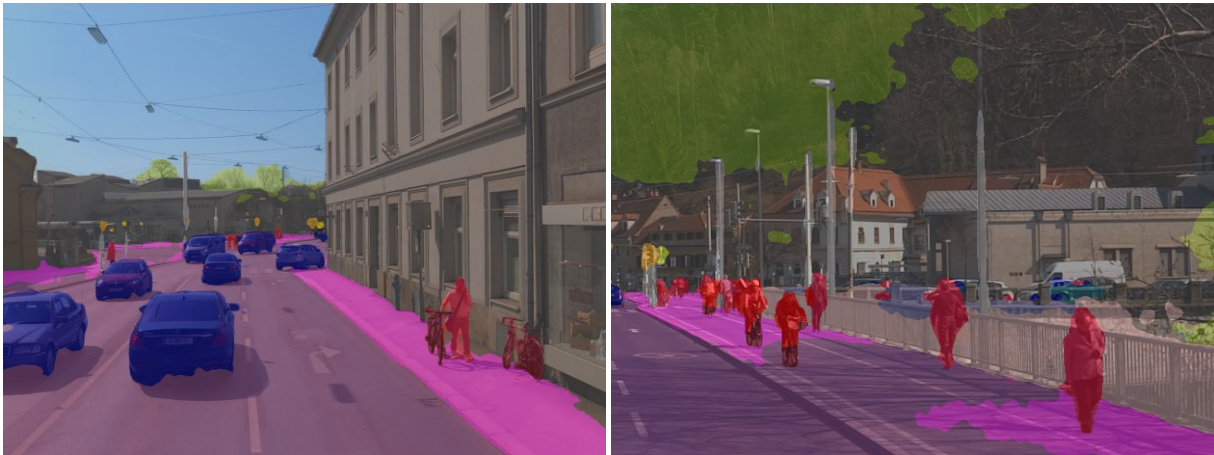
Fig. 2 Segmentation examples, classes are colour coded and overlaid onto the original RGB images. On the right side an example of failed segmentation is visible, parts of the sidewalk and bicycle lane are incorrectly classified as road
