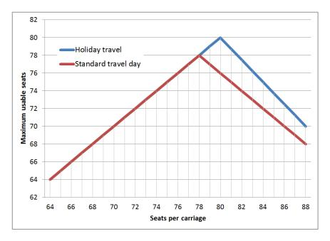
Figure 5: Maximum possible number of seats in passenger carriages with a length of 26.4 meters over buffers (Source: Rüger)
