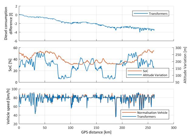
Fig. 6 Illustration of HoD operation; BOB test with 40 tonne GCW; speed profile mean standard deviation between normalization vehicle (Ref FH1758) and the Transformers vehicle under test:  $\sigma = 1.5$  km/h
