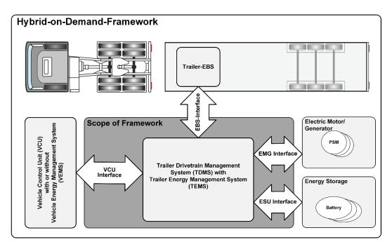
Fig. 3 Logical System Architecture of the HoD-Framework
