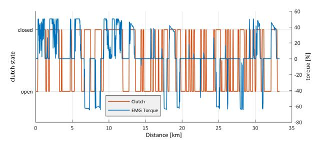
Fig. 7 Illustration of HoD clutch engagement and EMG torque variation; BOGA test with 40 GCW (negative torques correspond to braking and thus SoC increase)
