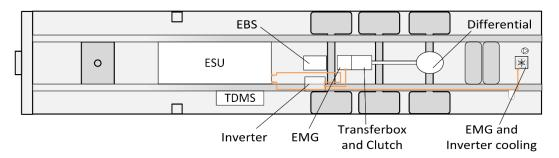
Fig. 4 Top View of the TRANSFORMERS trailer with the location of important components
