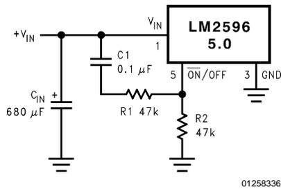
FIGURE 21. Delayed Startup
