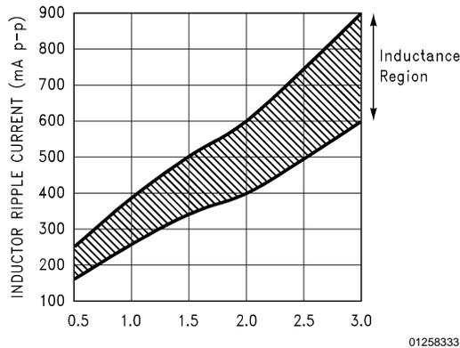
**FIGURE 18. Peak-to-Peak Inductor Ripple Current vs Load Current**
