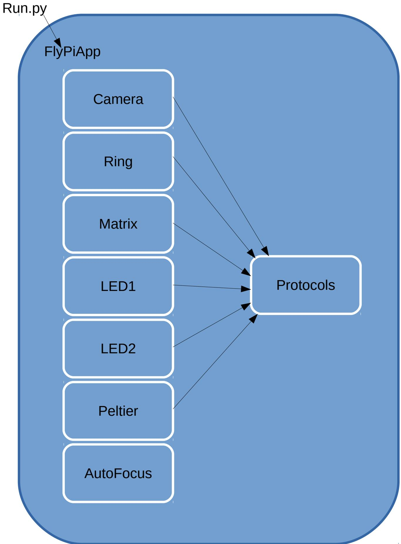
Software schematics – Flypi class contains all classes. Whenever the Protocol class is activated, the other activated classes are passed into Protocol.
