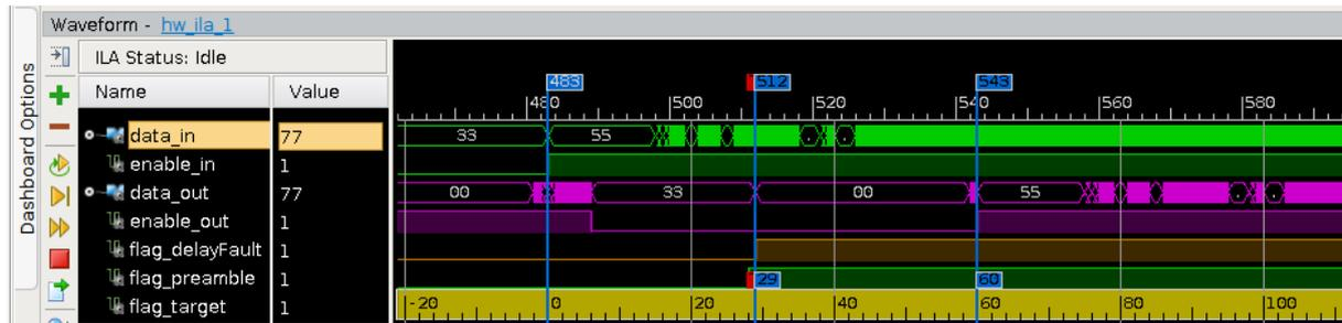
Fig. 5 ILA illustration for delay fault of 1 $\mu$ s
