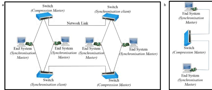
Fig. 1 (a) Multi-hop Redundant configuration for TTEthernet; (b) Single-hop non-redundant configuration for TTEthernet
