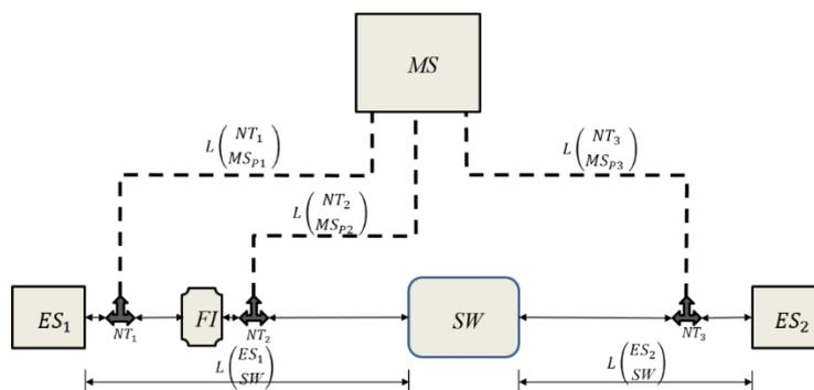
Fig. 3 Single Hop Non-redundant network connected to a monitoring station
