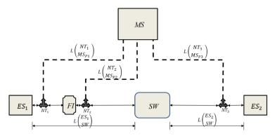
Fig. 3 Single Hop Non-redundant network connected to a monitoring station
