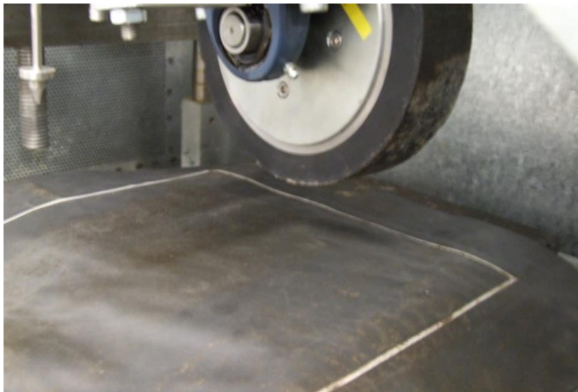
Figure 2. Test set-up with the small wheel track up and the flexible pressure mat over the sample
