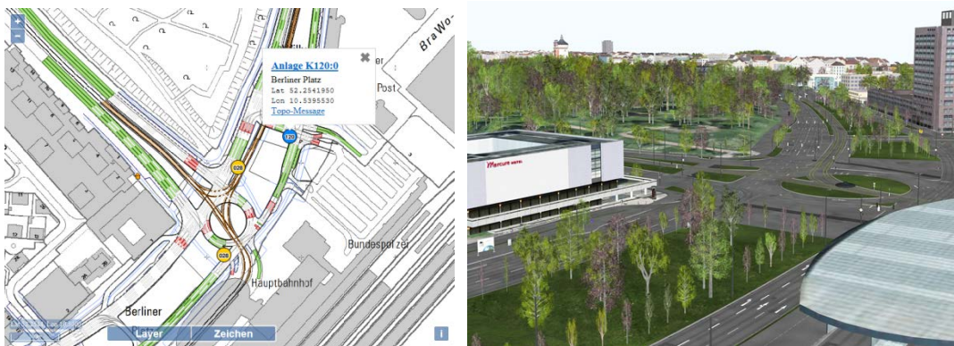
Figure 6: Visualization of different geodata (e.g. TOPO messages of intersection parts and road topography) contained by the Digital Atlas (left) and a generated 3D environment from the same intersection using various geodata hosted by the Digital Atlas (right).
