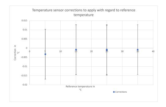
In the calibration conditions, the expanded uncertainty of the corrections to apply to the indications provided by the sensor (corrections not included in the uncertainty) is estimated to be:
