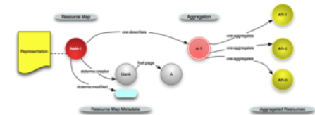
Open Archives Initiative Object Exchange and Reuse Aggregation to enumerate and link together
