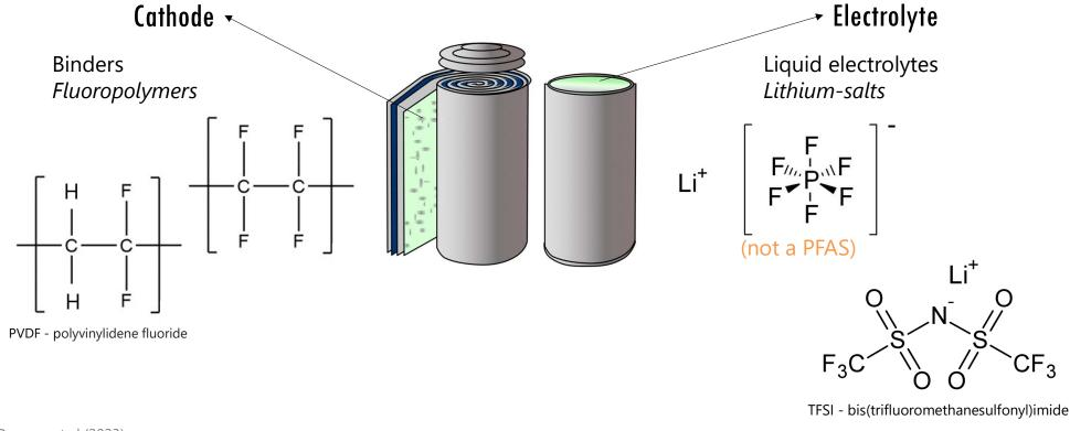
Rensmo et al (2023) Savvidou et al. (2024) "The inclusion of **fluorine-based compounds** in the electrolyte chemistry is, to date, ubiquitous as a pathway to promote the targeted formation of lithium fluoride, known to be a favourable SEI component in lithium batteries."
