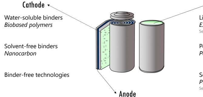
Styrene-Butadiene Rubber (SBR) Carboxymethylcellulose (CMC) Polyacrylic acid (PAA) - Electrolyte
