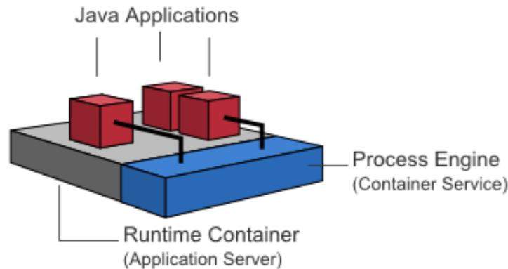
*Figure 7: Shared, Container-Managed Process Engine*
