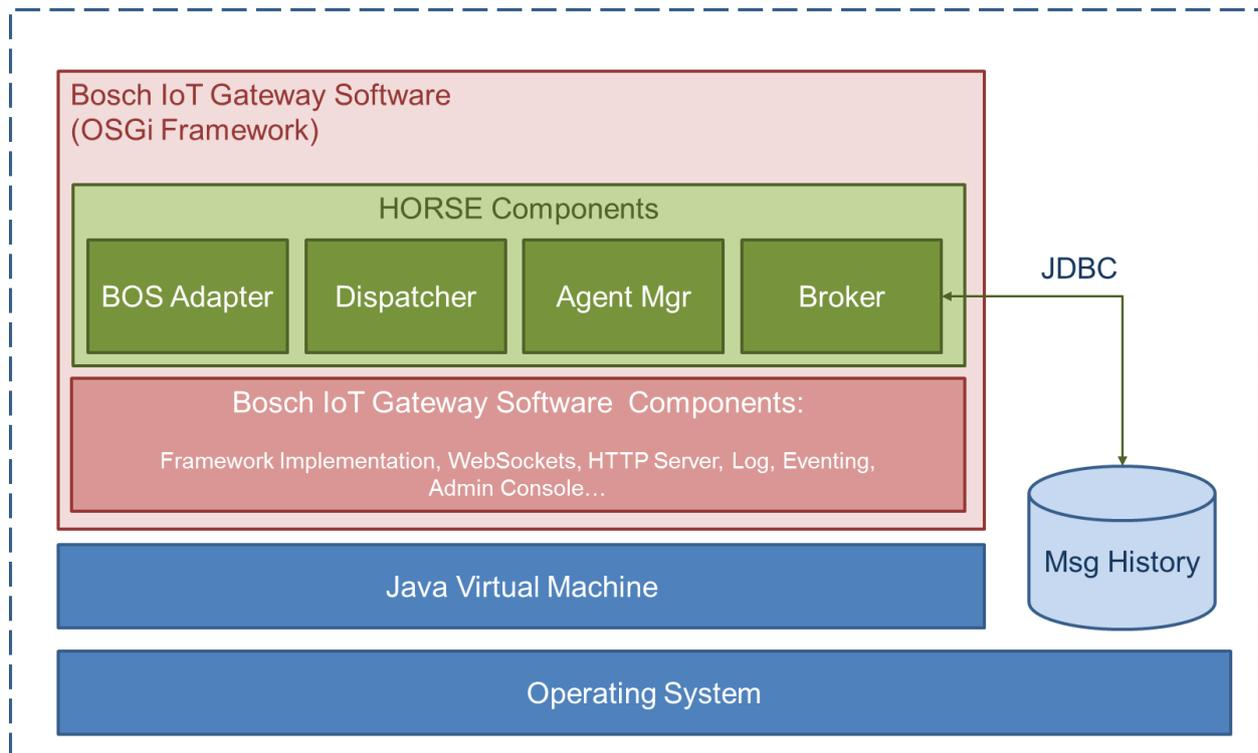
*Figure 5: Execution Environment for PRO modules*
