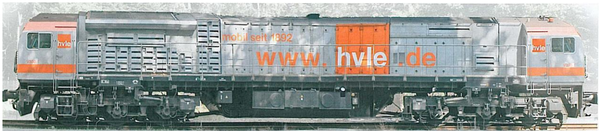
Figure 7. Refurbished Diesel locomotive of operator HVLE, Germany, power 2500 kW, traction force 517 kN, Vmax 120 km/h, mass 126 t, Length 23410 mm, 7 locos rebuilt since 2008
