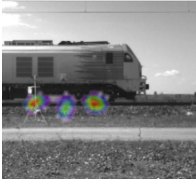
Figure. 8. Sound source localization for a Co'Co' locomotive under electric mode at 120 km/h and 2500 Hz
