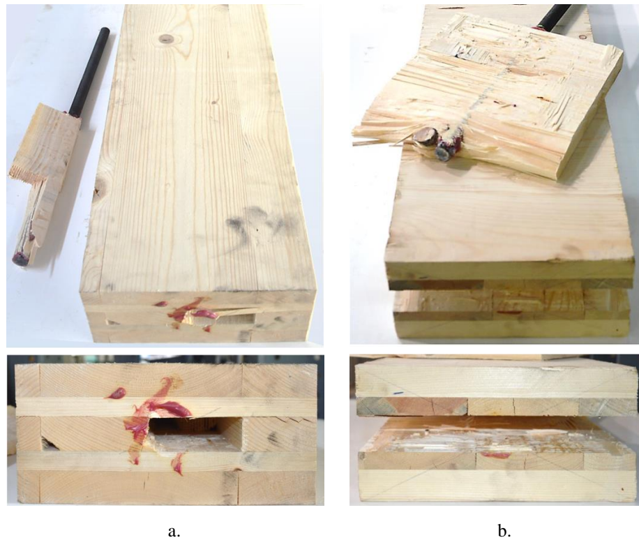
Fig. 4 Typical response of the specimens with l_a = 320 mm: a.) rod parallel to the grain and b.) rod perpendicular to the grain of the middle CLT layer
