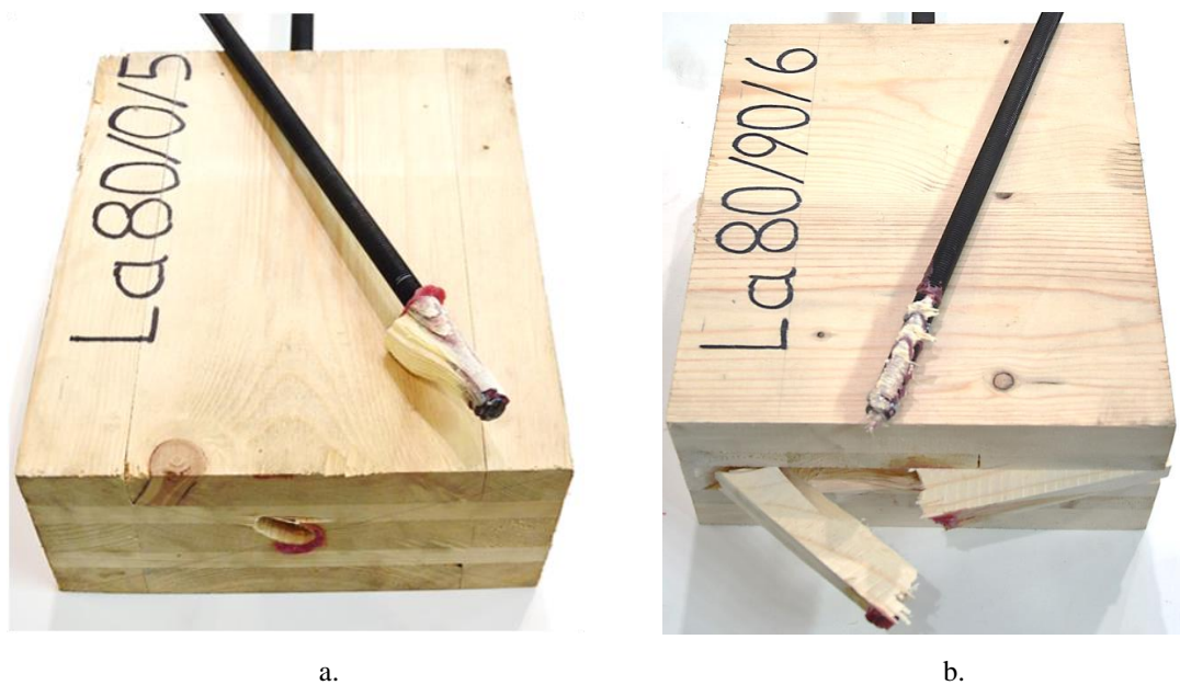
Fig. 2 Typical response of the specimens with l_a = 80 mm: a.) rod parallel to the grain and b.) rod perpendicular to the grain of the middle CLT layer
