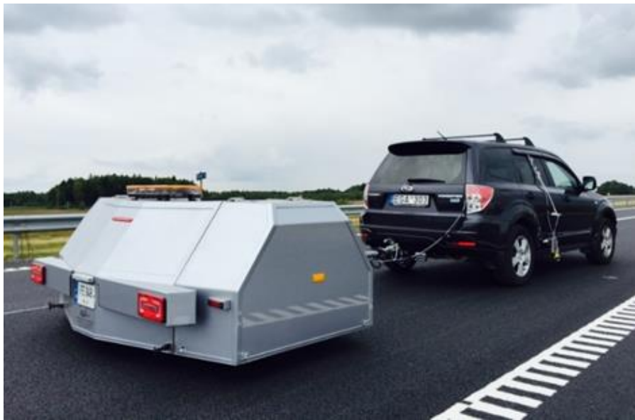
Fig. 2 CPX noise level measurement trailer.
