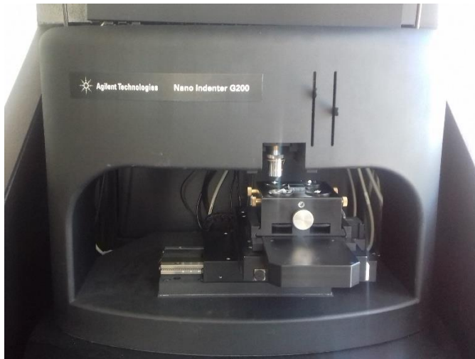
Fig. 1 Agilent Nano indenter G200 chamber
