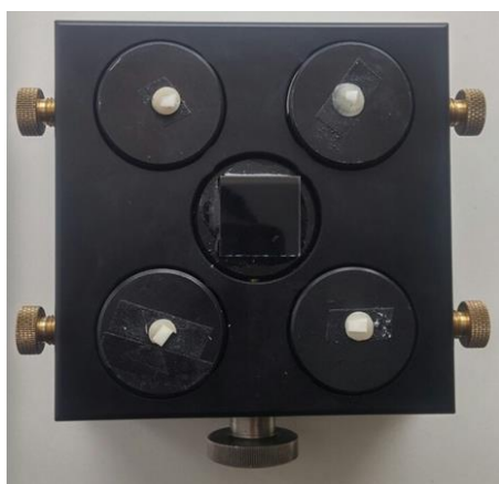
Fig. 2 Sample holder with four specimens obtained after cutting and polishing (fifth sample in the center of the holder is referent fused silica sample)
