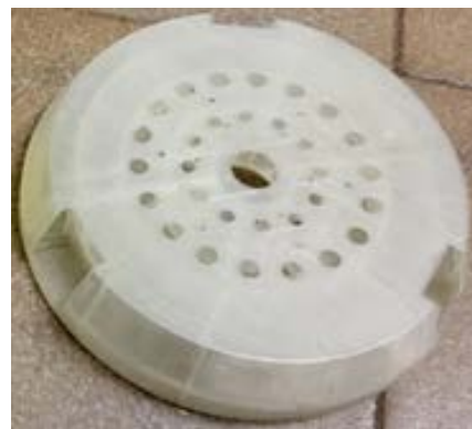
Figure 9: 3D printed strongback concept
