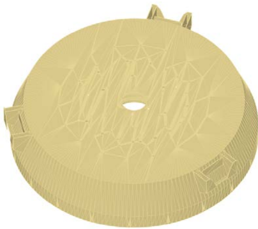
Figure 3: Strongback mesh structure for simulation with OpenFOAM
