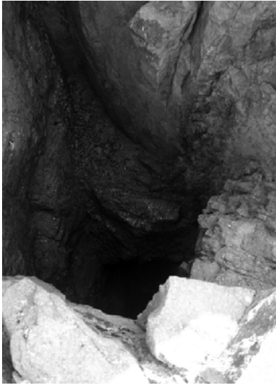
Figure 4a. The tunnels dug perpendicular to the ore body
